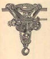
Swivel and reversiblebest used as a fork carrier but may be used as a sling carrier with proper self-locking sling pulleys having Ney No. RH24X registering head. Fork pulley has patented snap hook for safer lifting. Lifting pulleys lock directly on side or frame of carrier -not depending on separate dogs or lugs to hold the load.
