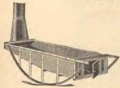
Made of cast iron and best quality sheet iron, he avily bound and riveted, strongly made. Mounted on rockers of heavy angle iron—thus furnishing a complete portable furnace of iron, yet light enough so it can be easily handled by two men.
